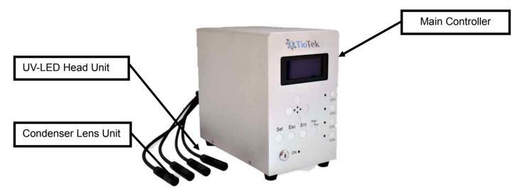
This product is a light source for ultraviolet light output using UV-LED for the light output source. The UV-LED included in the LED Head Unit outputs the light which is then applied to any place as desired. This equipment consists of the optical system including UV-LED with exchangeable condenser lens and controller. UV output can be executed by using the control switches or external control signals.
